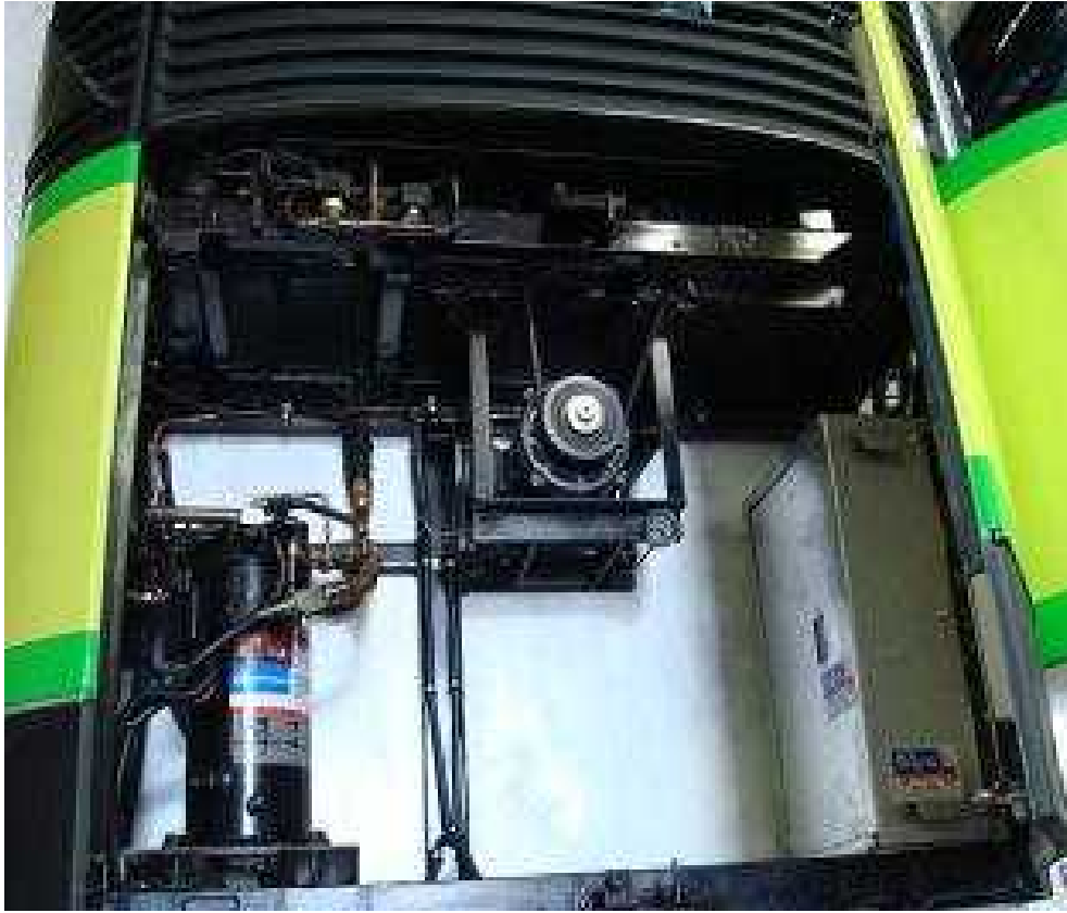
Demo eTRU using a Copeland Scroll Digital™ compressor and Intra-Tech's prototyped controller
