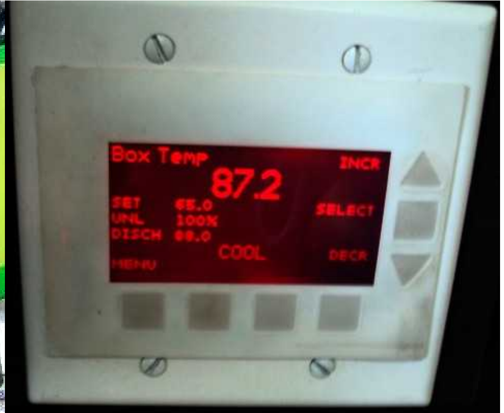
Intra-Tech's prototyped controller LCD display with membrane keys
